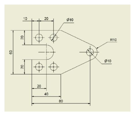
You are required to model the part described in the illustration shown above. Extrude the sketch by 10mm to create the solid model part.
